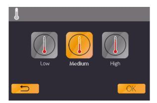
Low temperature: 85°C-87°C Medium temperature:87C -90°C High temperature: 90°C – 93°C
