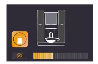
(Remarks: During the milk frother making process, users can press icon to stop the milk frother making process, then the coffee machine will continue to brew espresso.)
